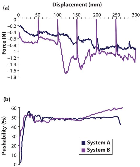
→ and Sample B. It is clear from Figure 2 (a) that the trackability force has decreased with a reduction in o.d. of the sample. The results of pushability tests conducted on the same samples along the same path are shown in Figure 2 (b). A 6% reduction in pushability was recorded when the o.d. was reduced by 7%.
