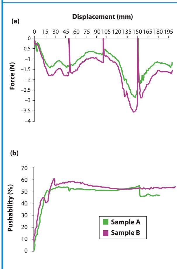
**Figure 3:** (a) Trackability and (b) pushability results obtained during benchmark testing of stent delivery system A and stent delivery system B.
