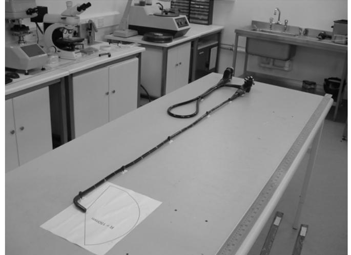
Figure 3: Endoscopic shape set resilience test jig (9).
