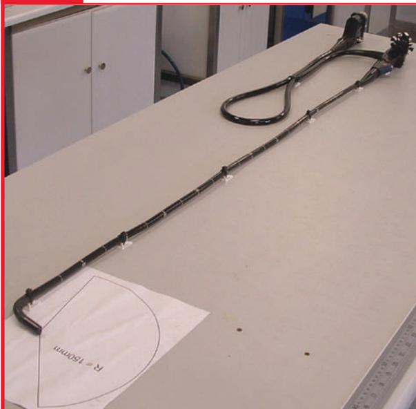
The needle was completely withdrawn from the endoscope and evaluated for permanent deformation.
